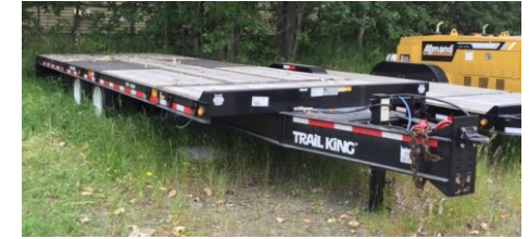
2015 Trail King TKT40LP Low Profile Tilt Trailer 40,000 lb. capacity, 12,000 lb. Spring Foot Jack 24' Tilt with 4' Stationary Deck Price includes F.E.T., Title and Licensing Fees Unit #U15024 - NEW
